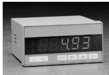
The Digital Monitor Model 2590 receives a  $4 \sim 20\text{mA}$  signal from the vibration converter, scales it into a vibration value for digital display and allows the vibration to be
