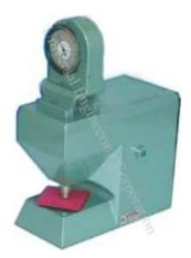
Used for rapid and accurate **measurement of thickness of paper, board and plastics.** Both Models are compact ones and measure thickness of paper, board, plastic films, rapidly and accurately. Measuring spindle with constant lowering speed (1mm/sec).
