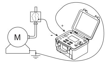
To measure high insulation values (> 1  $G\Omega$ ), we recommend using guard terminal "G" to avoid leakage and capacitive effects or eliminate the influence of surface leakage currents. The guard terminal is connected to a surface where leakage currents may flow through dust and humidity, e.g. the insulation surface of a cable or transformer, between two measurement points.
