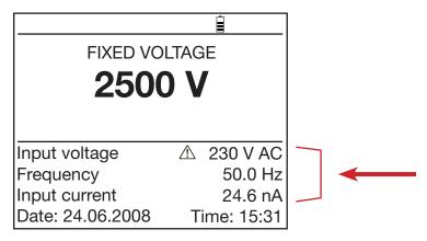
The insulation measurements cannot be started if there is an excessively high external voltage on the terminals, in which case the \(\begin{align\*} \text{Symbol} \) symbol is displayed next to the measured external voltage (see § 3.2).
