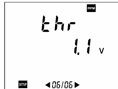
Figure 49: Display of parameter relating to the threshold voltage of the tachometer sensor.
