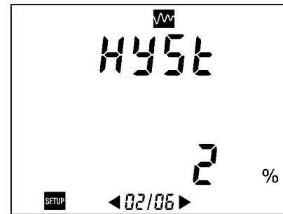
Figure 45: Display of parameter relating to hysteresis.
