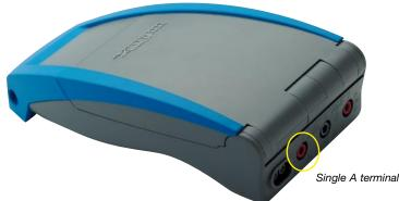
For greater efficiency and safety when working, the instrument proposes only 3 measurement terminals.
