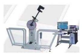
A impact testing machine is used to determine the energy absorbed in fracturing a test piece at high velocity. JB-W300A computer controlled impact tester can not only examine the energy, return zero, loss of energy, swing circle, but also can display, store, print the testing result through computer. You can control it by computer software or control box. With 300J and 150J pendulums separately, this machine can examine the impact energies at high precise.
