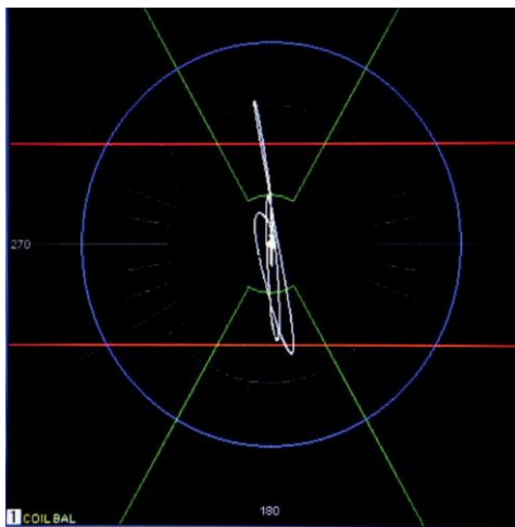
Minimac EC screen polar view of thresholds with a test signal for a drilled hole in a copper tube.
