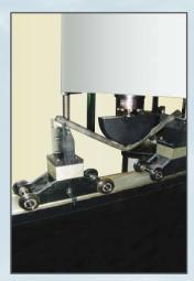
Bending test attachment for automobile bumper
