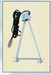
Small deformation extensometer
