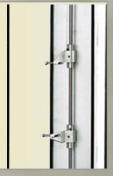
High deformation extensometer
