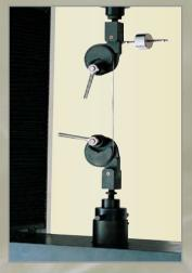
Steel wire winding tension grip
