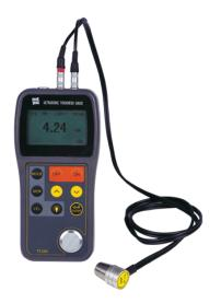
Time Group ultrasonic thickness gauges measure the thickness of ultrasonic wave wellconductive materials with parallel top and bottom surfaces. It measures the thickness of both metal (steel, aluminum, titanium, etc.) and nonmetal (plastics, ceramics, glass, etc.) parts. They are commonly used to measure (remaining) wall thickness of pipes and pressure vessels.
