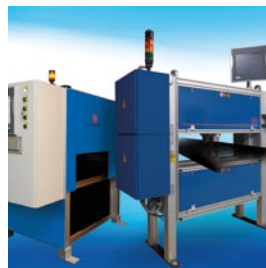
Profilometer for thickness measurement of running surfaces and side walls Page 8-9
