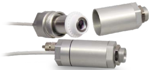
Dirt and deposit on the lens like smoke, steam and high air humidity (condensation) are avoided or reduced by using an air purge collar.
