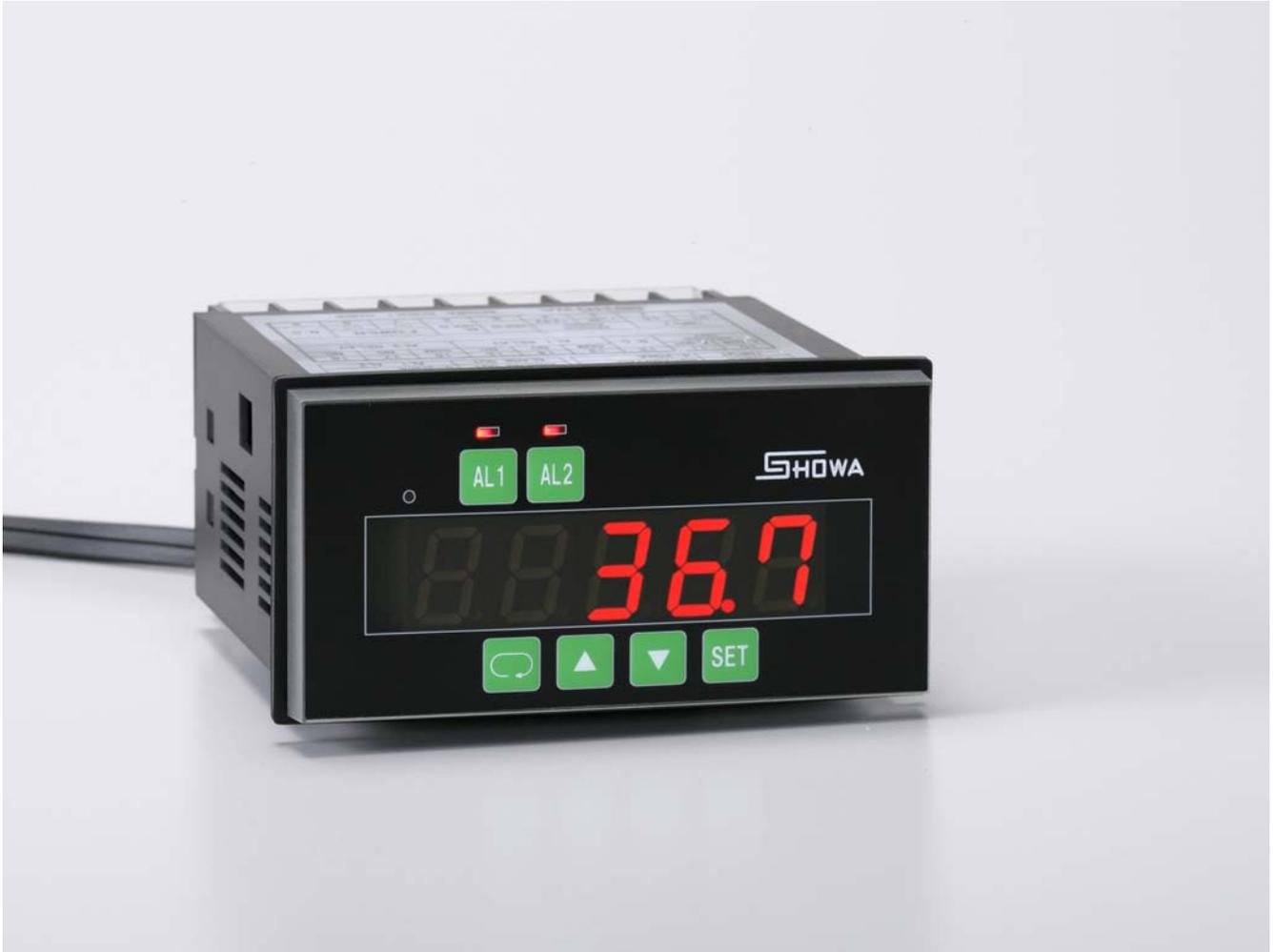
**In combination with any of the vibration converters, Vibro Converter 2502 Series, this digital allows you to measure and monitor vibrations easily.**
