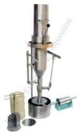
For production of laboratory sheets for physical tests. The design of the drainage system provides a uniform flow across the entire wire, thus permitting exceptionally uniform sheets.
