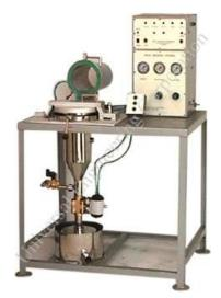
Semi-Automated Sheet Former For producing the pulp sheet rapidly for physical strength tests. In comparison to the standard sheet former, this apparatus reduces the time factor, increases the output, improves the reproducibility, reduces the operator's influence and fatigue without effecting to the final product. Stirring in the apparatus is an automatic function by use of compressed air, whilst couching is effected by means of pneumatic fixture.
