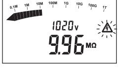
During measurements the instrument will beep every 10 seconds to alert the user that a high voltage is present.
