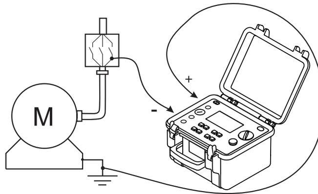
**To measure high insulation values (> 1 GΩ),** we recommend using guard terminal “G” to avoid leakage and capacitive effects or eliminate the influence of surface leakage currents. The guard terminal is connected to a surface where leakage currents may flow through dust and humidity, e.g. the insulation surface of a cable or transformer, between two measurement points.
