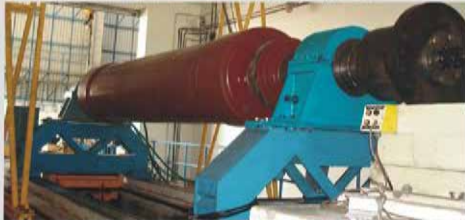
A 32 ton generator rotor being balanced at operating speed of 1000 rpm on ABRO HR25K machine
