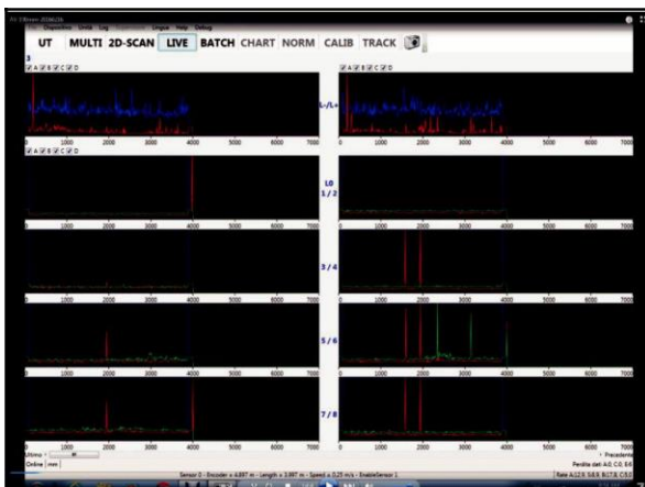
Echomac 180 PA live screen display of a calibration standard with defects.
