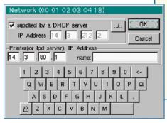
It is really simple to configure communications because, in most cases, the instrument's IP address is supplied automatically by the local server. All you have to do is enter the address of the printer to be used.
