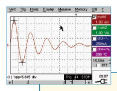
Many complex functions are editable, including simulation of a trace on the basis of its mathematical equation and therefore modelling of an expected result. There is almost infinite capacity for saving the functions created so that they can be recalled subsequently.
