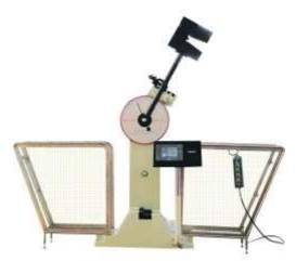
A impact testing machine is used to determine the energy absorbed in fracturing a test piece at high velocity. JB-S300A digital display touchscreen type impact tester can not only examine the energy, return zero, loss of energy, swing circle, but also can display, store, print the testing result through a microcomputer. You can control it by touch screen or by control box. With 300J and 150J pendulums separately, this machine can examine the impact energies at high precise.
