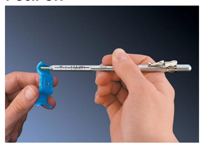
Measures non-magnetic coatings such as paint, enamel, plating, hot-dip galvanizing on steel.
