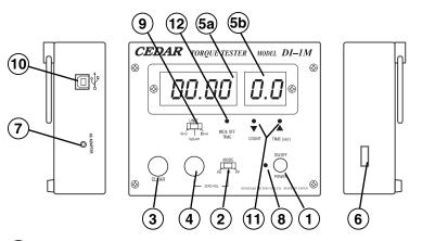
**ON/OFF Switch** Press to turn on, press again to turn off (click (1) once, do not hold). After 10 minutes of non-use the unit shuts off.
