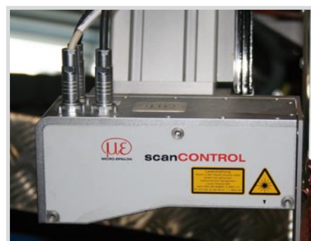
The laser line sensors provide exact profile data on the weld seam profile.
