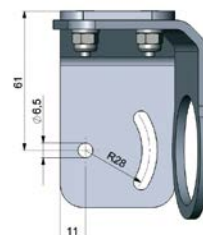
TM-AB-CTL Mounting bracket (adjustable)
